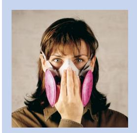
Place the palm of your hand over the exhalation valve cover and exhale gently. The facepiece should bulge slightly. If air leaks between the face and the faceseal of the respirator, reposition it and adjust the straps for a more secure seal.\*
